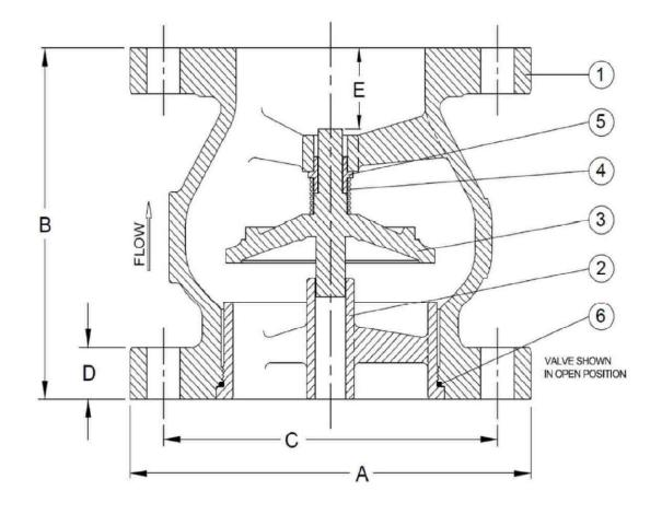
SEE DRAWING NO. VM-1800A-M-AND 3748-M FOR MATERIALS OF CONSTRUCTION
